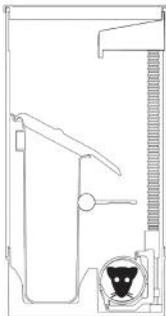
2. The elevator lifts the rodent upwards where it receives an electric charge.
